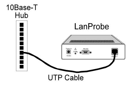
Figure 3-14: Connecting LanProbe to 10Base-T Networks
